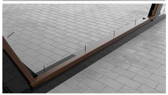
• Next, install the center wooden batten (45x95 mm), which can be screwed into the previously secured battens, and the short diagonal batten (45x45 mm) to secure the overhanging ends. Use 5x90 mm wood screws for fastening.
