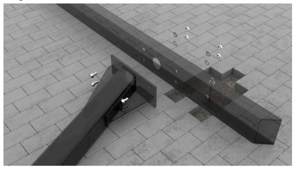
• Use M20 bolts, nuts, and washers to secure the connections, with 4 sets of each for every corner post (CP-1; CP-2; CP-3; CP-4).
