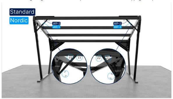
• Install the inner ridge diagonal plates using 3 pcs of M10x25 bolts and 2 pcs of SFS TDBL-10.6 self-tapping bolts per plate.
