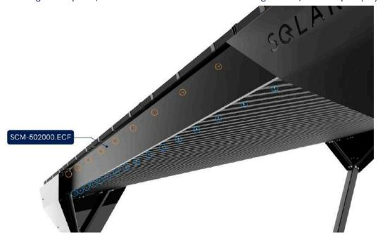
• To cover the outer diagonal plates of the eave, install the cover flashings and secure them using DIN 7504-K 5.5x32mm Self-Drilling Screws, A2 + Ruspert (C3).
