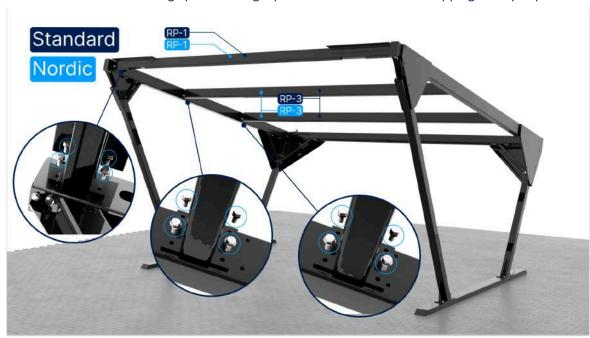
• Install the ridge diagonal braces with 12 pcs of SFS TDBL-13.4 self-tapping bolts per brace.
