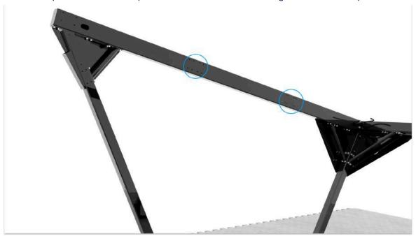
• For the FRS G2.5 BIPV panel, select the lower set of holes to secure the middle two purlins, and for the FRS G3 BIPV panel, select the upper set.
