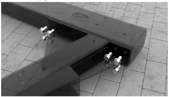
• Secure the wall diagonal braces (<u>Standard</u> and <u>Nordic</u>) using 8 pcs of SFS TDBL-13.4 self-tapping bolts for each brace.
