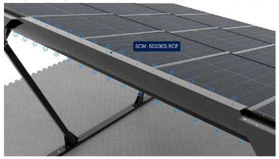
• To cover the outer ridge diagonal plates, install the cover flashings. For fastening from the top of the roof, use 4.8x35 KAT.KR/6K BLACK-250-4. For securing to the diagonal plate, use DIN 7504-K 5.5x32mm Self-Drilling Screws, A2 + Ruspert (C3).
