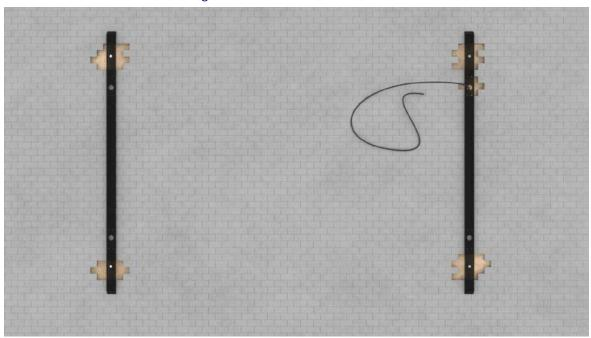
• Pull power cables through base rail (BR-1), corner post (CP-4) and roof beam (RB-1 or RB-2) before fastening the structural parts together.
