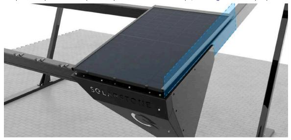
• Install the next 4 first-row panels in the same way, following the first-row clamps, and ensure that the weather lock is in the closed position. The left edge of the panel row must end flush with the metal structure.
