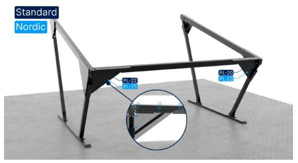
• Install the outer diagonal plates using 3 pcs of M10x25 bolts and 2 pcs of SFS TDBL-10.6 self-tapping bolts.
